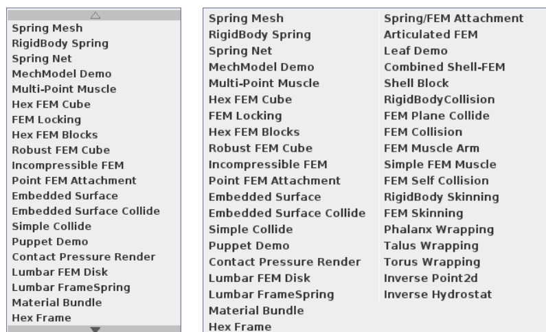
Figure 60: When the number of menu entries exceeds the maximum number of rows, either a scrolling menu is used if scrolling is enabled (left), or additional columns are added to the menu (right).
